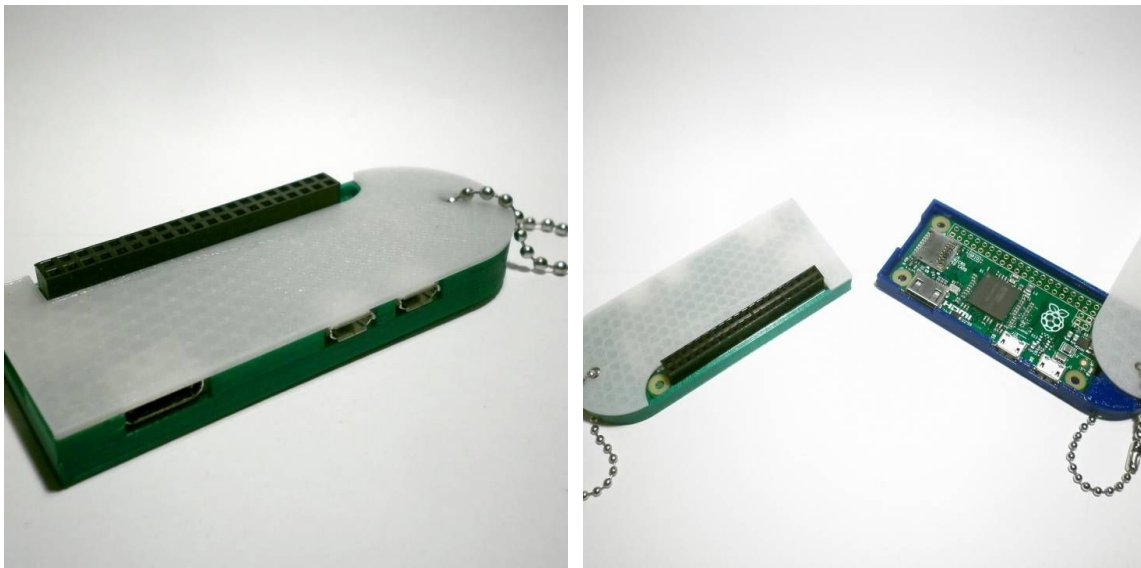
Figure 30. Initial outlook of the 3D-printed case without the microphone array
